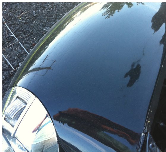
Figure 6. Black is the most difficult color to match an automobile. Over time the smooth surface develops microscopic pitting that creates highlights and shadows, thereby weakening the pure black appearance.
